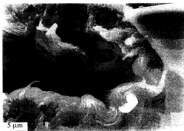
Figure 7 SEM micrograph of the stopped crack front in the Izod impact test, recorded from the side view as shown in Figure 4 . Extensive folding of the flank surface layer and buckling of the elongated cavities are readily discernible
